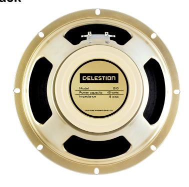
The new G10 Creamback packs everything guitar players love about Creamback speakers into a 10-inch format. Hand-built in the UK using the same production methods and materials developed for the 12-inch models, the G10 Creamback uses a ceramic magnet and a 1.75-inch voice coil to deliver 45-watt power handling. With all the punch and dynamics typical of a 10 its overall tone is warm expressive detailed and well-balanced.
