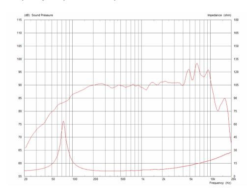
Power rating: Tested for two hours using a continuous, band-limited pink noise signal as per AES standard. Power calculated on minimum impedance. Loudspeaker tested in free air. Continuous power rating: Defined as 3dB greater than the AES rating. Sensitivity: Measured on axis at 1W, 1m in 2 anechoic environment. Parameters: Measured after unit subjected to
